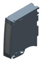
SIMATIC S7-1500 Analog input module, AI 8xU/I/R/RTD BA, 16 bit resolution, Accuracy 0.5%, 8 channels in groups of 8; Common mode voltage 4 V DC, Diagnostics; Hardware interrupts; Delivery including infeed element, shield bracket and shield terminal: Front connector (screw terminals or push-in) to be ordered separately
