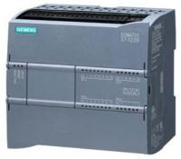
SIMATIC S7-1200, CPU 1214C, compact CPU, AC/DC/relay, onboard I/O: 14 DI 24 V DC; 10 DO relay 2 A; 2 Al 0-10 V DC, power supply: AC 85-264 V AC at 47-63 Hz, program/data memory 150 KB
