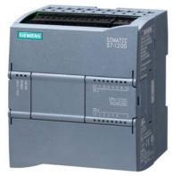
SIMATIC S7-1200, CPU 1212C, compact CPU, DC/DC/DC, onboard I/O: 8 DI 24 V DC; 6 DO 24 V DC; 2 AI 0-10 V DC, power supply: DC 20.4-28.8 V DC, program/data memory 100 KB
