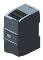
SIPLUS S7-1200 SM 1232 2AQ based on 6ES7232-4HB32-0XB0 with conformal coating, -20...+60 °C, analog output +/-10 V: 14-bit resolution or 0-20 mA: 13-bit resolution
