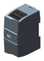
SIPLUS S7-1200 SM 1221 8DI based on 6ES7221-1BF32-0XB0 with conformal coating, -40...+70  $^{\circ}\text{C}$ , start up -25  $^{\circ}\text{C}$ , digital input 8 DI, 24 V DC, sink/source
