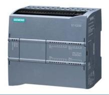
SIPLUS S7-1200 CPU 1214C AC/DC/relay based on 6ES7214-1BG40-0XB0 with conformal coating, -40...+70 °C, start up -25 °C, signal board: 0, compact CPU, AC/DC/relay, onboard I/O: 14 DI 24 V DC 10 DQ relay 2 A 2 AI 0-10 V DC, power supply: AC 85-264 V AC @ 47-63 Hz, program/data memory 100 KB
