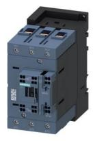
power contactor, AC-3e/AC-3, 110 A, 55 kW / 400 V, 3-pole, 230 V AC, 50 Hz, auxiliary contacts: 1 NO + 1 NC, main circuit: screw terminal, control and auxiliary circuit: spring-loaded terminal, size: S3  $\,$
