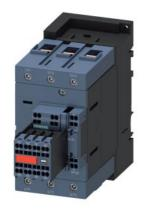
power contactor, AC-3e/AC-3, 95 A, 45 kW / 400 V, 3-pole, 20-33 V AC/DC, 50/60 Hz, with integrated varistor, auxiliary contacts: 2 NO + 2 NC, main circuit: screw terminal, control and auxiliary circuit: spring-loaded terminal, size: S3, captive auxiliary switch
