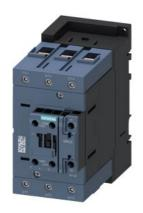
power contactor, AC-3e/AC-3, 95 A, 45 kW / 400 V, 3-pole, 24 V DC, 0.8-1.2\* Us, with integrated varistor, auxiliary contacts: 1 NO + 1 NC, screw terminal, size: S3, suitable for PLC outputs, upright mounting position
