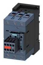
power contactor, AC-3e/AC-3, 95 A, 45 kW / 400 V, 3-pole, 230 V AC, 50/60 Hz, with plugged-in varistor, auxiliary contacts: 2 NO + 2 NC, screw terminal, size: S3, captive auxiliary switch
