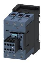
power contactor, AC-3e/AC-3, 95 A, 45 kW / 400 V, 3-pole, 400 V AC, 50 Hz, auxiliary contacts: 2 NO + 2 NC, screw terminal, size: S3, removable auxiliary switch
