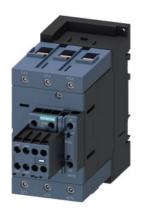
power contactor, AC-3e/AC-3, 95 A, 45 kW / 400 V, 3-pole, 110 V AC, 50 Hz / 120 V, 60 Hz, auxiliary contacts: 2 NO + 2 NC, screw terminal, size: S3, removable auxiliary switch
