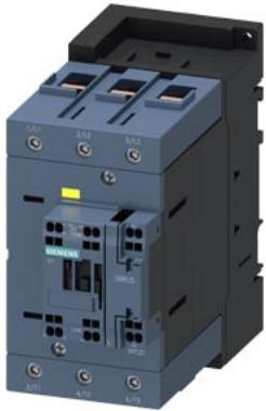
power contactor, AC-3e/AC-3, 80 A, 37 kW / 400 V, 3-pole, 21-33 V AC/DC, 50/60 Hz, with integrated varistor, auxiliary contacts: 1 NC, main circuit: screw terminal, control and auxiliary circuit: spring-loaded terminal, size: S3, F-PLC-IN
