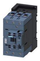
power contactor, AC-3e/AC-3, 80 A, 37 kW / 400 V, 3-pole, 83-155 V AC/DC, 50/60 Hz, with integrated varistor, auxiliary contacts: 1 NO + 1 NC, main circuit: screw terminal, control and auxiliary circuit: spring-loaded terminal, size: S3
