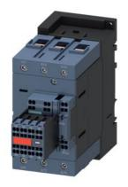
power contactor, AC-3e/AC-3, 80 A, 37 kW / 400 V, 3-pole, 20-33 V AC/DC, 50/60 Hz, with integrated varistor, auxiliary contacts: 2 NO + 2 NC, main circuit: screw terminal, control and auxiliary circuit: spring-loaded terminal, size: S3, captive auxiliary switch
