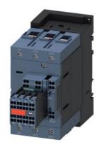
power contactor, AC-3e/AC-3, 80 A, 37 kW / 400 V, 3-pole, 24 V DC, 0.8-1.2\* Us, with integrated varistor, auxiliary contacts: 1 NO + 1 NC, integrated varistor, main circuit: screw terminal, control and auxiliary circuit: spring-loaded terminal, size: S3, suitable for PLC outputs, captive auxiliary switch
