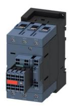
power contactor, AC-3e/AC-3, 80 A, 37 kW / 400 V, 3-pole, 230 V AC, 50 Hz, with plugged-in varistor, auxiliary contacts: 2 NO + 2 NC, main circuit: screw terminal, control and auxiliary circuit: spring-loaded terminal, size: S3, captive auxiliary switch
