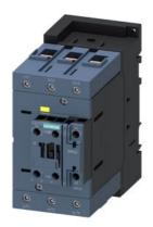
power contactor, AC-3e/AC-3, 80 A, 37 kW / 400 V, 3-pole, 175-280 V AC/DC, 50/60 Hz, with integrated varistor, auxiliary contacts: 1 NC, screw terminal, size: S3, F-PLC-IN
