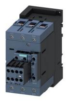
power contactor, AC-3e/AC-3, 80 A, 37 kW / 400 V, 3-pole, 175-280 V AC/DC, 50/60 Hz, with integrated varistor, auxiliary contacts: 2 NO + 2 NC, screw terminal, size: S3, removable auxiliary switch
