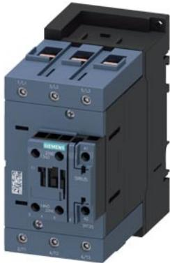
power contactor, AC-3e/AC-3, 80 A, 37 kW / 400 V, 3-pole, 20-33 V AC/DC, 50/60 Hz, with integrated varistor, auxiliary contacts: 1 NO + 1 NC, screw terminal, size: S3
