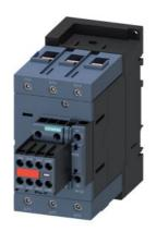
power contactor, AC-3e/AC-3, 80 A, 37 kW / 400 V, 3-pole, 24 V DC, 0.8-1.2\* Us, with integrated varistor, auxiliary contacts: 1 NO + 1 NC, screw terminal, size: S3, suitable for PLC outputs, captive auxiliary switch
