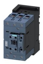
power contactor, AC-3e/AC-3, 80 A, 37 kW / 400 V, 3-pole, 220 V AC, 50 Hz / 264 V, 60 Hz, auxiliary contacts: 1 NO + 1 NC, screw terminal, size: S3  $\,$
