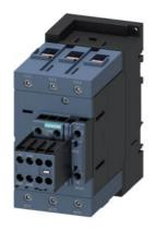
power contactor, AC-3e/AC-3, 80 A, 37 kW / 400 V, 3-pole, 24 V AC, 50 Hz, auxiliary contacts: 2 NO + 2 NC, screw terminal, size: S3, removable auxiliary switch
