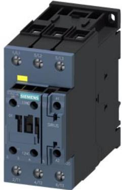
power contactor, AC-3e/AC-3, 80 A, 37 kW / 400 V, 3-pole, 83-150 V AC/DC, 50/60 Hz, with integrated varistor, auxiliary contacts: 1 NC, screw terminal, size: S2, F-PLC-IN
