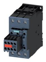
power contactor, AC-3e/AC-3, 80 A, 37 kW / 400 V, 3-pole, 20-33 V AC/DC, 50/60 Hz, with integrated varistor, auxiliary contacts: 2 NO + 2 NC, screw terminal, size: S2, captive auxiliary switch
