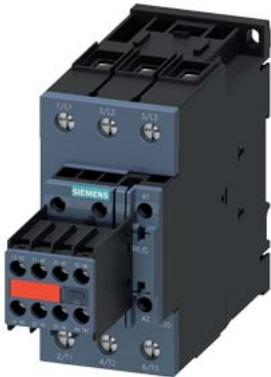
power contactor, AC-3e/AC-3, 80 A, 37 kW / 400 V, 3-pole, 110 V AC, 50 Hz / 120 V, 60 Hz, with plugged-in varistor, auxiliary contacts: 2 NO + 2 NC, screw terminal, size: S2, captive auxiliary switch
