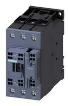
power contactor, AC-3e/AC-3, 65 A, 30 kW / 400 V, 3-pole, 230 V AC, 50/60 Hz, with plugged-in RC element, auxiliary contacts: 1 NO + 1 NC, main circuit: screw terminal, control and auxiliary circuit: spring-loaded terminal, size: S2,
