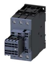
power contactor, AC-3e/AC-3, 65 A, 30 kW / 400 V, 3-pole, 110 V AC, 50 Hz, auxiliary contacts: 2 NO + 2 NC, main circuit: screw terminal, control and auxiliary circuit: spring-loaded terminal, size: S2, removable auxiliary switch
