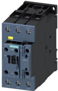
power contactor, AC-3e/AC-3, 65 A, 30 kW / 400 V, 3-pole, 83-150 V AC/DC, 50/60 Hz, with integrated varistor, auxiliary contacts: 1 NC, screw terminal, size: S2, F-PLC-IN
