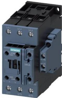
power contactor, AC-3e/AC-3, 65 A, 30 kW / 400 V, 3-pole, 20-33 V AC/DC, 50/60 Hz, with integrated varistor, auxiliary contacts: 2 NO + 2 NC, screw terminal, size: S2, lateral auxiliary switch
