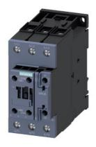
power contactor, AC-3e/AC-3, 65 A, 30 kW / 400 V, 3-pole, 20-33 V AC/DC, 50/60 Hz, with integrated varistor, auxiliary contacts: 1 NO + 1 NC, screw terminal, size: S2, upright mounting position
