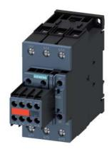
power contactor, AC-3e/AC-3, 65 A, 30 kW / 400 V, 3-pole, 230 V AC, 50/60 Hz, with plugged-in varistor, auxiliary contacts: 2 NO + 2 NC, screw terminal, size: S2, captive auxiliary switch
