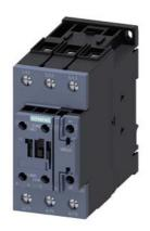
power contactor, AC-3e/AC-3, 65 A, 30 kW / 400 V, 3-pole, 230 V AC, 50/60 Hz, auxiliary contacts: 1 NO + 1 NC, screw terminal, size: S2, upright mounting position
