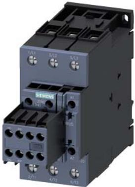
power contactor, AC-3e/AC-3, 65 A, 30 kW / 400 V, 3-pole, 110 V AC, 50 Hz / 120 V, 60 Hz, auxiliary contacts: 2 NO + 2 NC, screw terminal, size: S2, removable auxiliary switch
