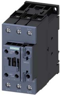
power contactor, AC-3e/AC-3, 65 A, 30 kW / 400 V, 3-pole, 110 V AC, 50 Hz / 120 V, 60 Hz, auxiliary contacts: 1 NO + 1 NC, screw terminal, size: S2, upright mounting position
