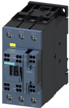
power contactor, AC-3e/AC-3, 51 A, 22 kW / 400 V, 3-pole, 21-33 V AC/DC, 50/60 Hz, with integrated varistor, auxiliary contacts: 1 NC, main circuit: screw terminal, control and auxiliary circuit: spring-loaded terminal, size: S2, F-PLC-IN
