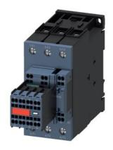
power contactor, AC-3e/AC-3, 51 A, 22 kW / 400 V, 3-pole, 24 V DC,  $0.8-1.2^{\circ}$  Us, with integrated varistor, auxiliary contacts: 2 NO + 2 NC, main circuit: screw terminal, control and auxiliary circuit: spring-loaded terminal, size: S2, suitable for PLC outputs, captive auxiliary switch
