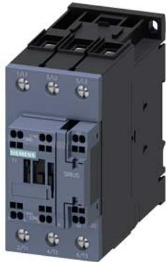
power contactor, AC-3e/AC-3, 51 A, 22 kW / 400 V, 3-pole, 230 V AC, 50/60 Hz, with plugged-in RC element, auxiliary contacts: 1 NO + 1 NC, main circuit: screw terminal, control and auxiliary circuit: spring-loaded terminal, size: S2,
