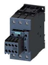
power contactor, AC-3e/AC-3, 51 A, 22 kW / 400 V, 3-pole, 24 V DC, 0.8-1.2\* Us, with integrated varistor, auxiliary contacts: 2 NO + 2 NC, screw terminal, size: S2, suitable for PLC outputs, removable auxiliary switch
