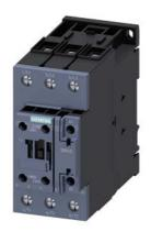
contactor, NEMA version, 25 HP, 460 / 575 V, 3-pole, 208 V AC, 50/60 Hz, auxiliary contacts: 1 NO + 1 NC, screw terminal, size: S2  $\,$
