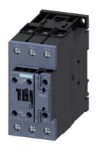
power contactor, AC-3e/AC-3, 51 A, 22 kW / 400 V, 3-pole, 110 V AC, 50 Hz, auxiliary contacts: 1 NO + 1 NC, screw terminal, size: S2, upright mounting position
