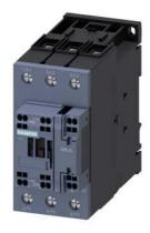
power contactor, AC-3e/AC-3, 41 A, 18.5 kW / 400 V, 3-pole, 400 V AC, 50 Hz / 400-440 V, 60 Hz, auxiliary contacts: 1 NO + 1 NC, main circuit: screw terminal, control and auxiliary circuit: spring-loaded terminal, size: S2,
