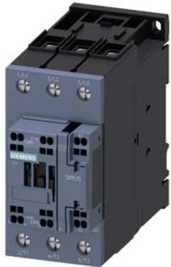
power contactor, AC-3e/AC-3, 41 A, 18.5 kW / 400 V, 3-pole, 24 V AC, 50 Hz, auxiliary contacts: 1 NO + 1 NC, main circuit: screw terminal, control and auxiliary circuit: spring-loaded terminal, size: S2, upright mounting position
