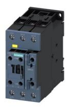
power contactor, AC-3e/AC-3, 41 A, 18.5 kW / 400 V, 3-pole, 83-150 V AC/DC, 50/60 Hz, with integrated varistor, auxiliary contacts: 1 NC, screw terminal, size: S2, F-PLC-IN
