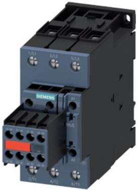
power contactor, AC-3e/AC-3, 41 A, 18.5 kW / 400 V, 3-pole, 20-33 V AC/DC, 50/60 Hz, with integrated varistor, auxiliary contacts: 2 NO + 2 NC, screw terminal, size: S2, captive auxiliary switch
