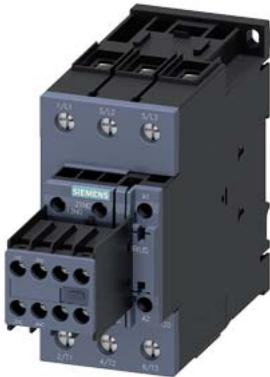
power contactor, AC-3e/AC-3, 41 A, 18.5 kW / 400 V, 3-pole, 230 V AC, 50 Hz, with plugged-in varistor, auxiliary contacts: 2 NO + 2 NC, screw terminal, size: S2, removable auxiliary switch
