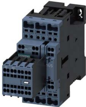
power contactor, AC-3e/AC-3, 38 A, 18.5 kW / 400 V, 3-pole, 24 V DC, auxiliary contacts: 2 NO + 2 NC, spring-loaded terminal, size: S0, removable auxiliary switch, reusable packaging, pack = 40 units
