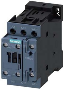
power contactor, AC-3e/AC-3, 38 A, 18.5 kW / 400 V, 3-pole, 220 V DC, auxiliary contacts: 1 NO + 1 NC, screw terminal, size: S0, India 40 A, Tu max. 50 °C
