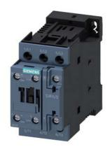
power contactor, AC-3e/AC-3, 38 A, 18.5 kW / 400 V, 3-pole, 24 V DC, auxiliary contacts: 1 NO + 1 NC, screw terminal, size: S0, upright mounting position
