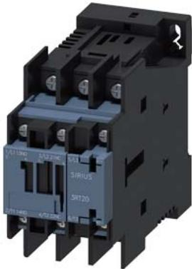
power contactor, AC-3e/AC-3, 32 A, 15 kW / 400 V, 3-pole, 24 V DC, 0.7-1.25\* Us, with plugged-in diode combination, auxiliary contacts: 1 NO + 1 NC, ring cable lug connection, size: S0
